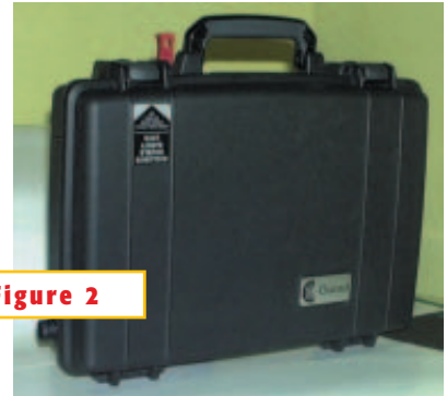
Netline's high-powered C-Guard HP has an effective jamming range of 20 to 1000m, depending on base-station-signal strength.
