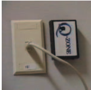
Figure 3 The Q-zone uses Bluetooth communications to signal compatible phones to switch to vibrating mode when they are in a quiet zone.
